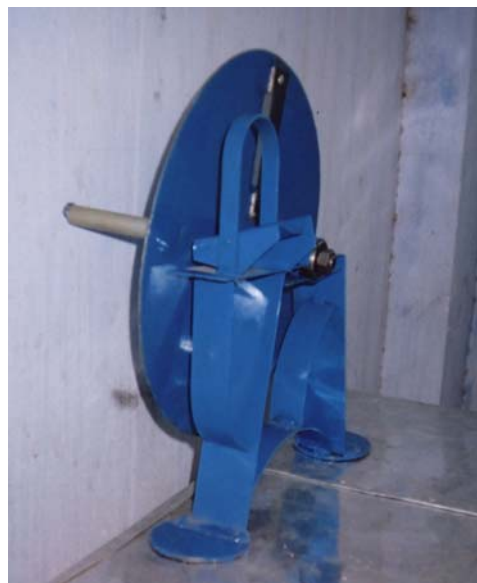
Fig. 2. Manual Cassava slicing implement
