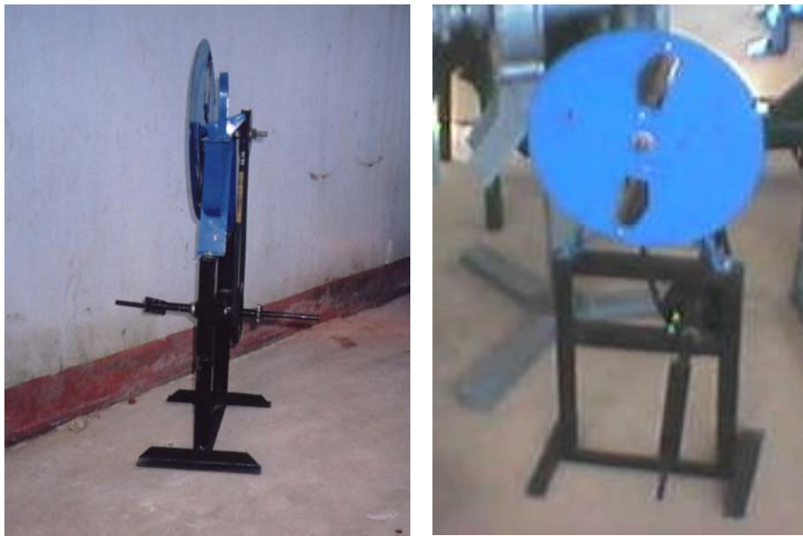
Fig. 4 Cassava pedal slicing implement
